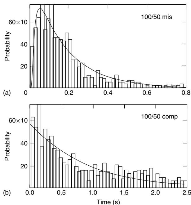
**Figure 5** Dwell time distributions of unzipping events of a 50/100 DNA hybrid, with 6-base mismatch (top) and perfect match (bottom). The mismatch events yield a characteristic timescale shorter by roughly a factor of 2 (185 ms vs. 435 ms). (Reproduced with permission from Ref. 32).
