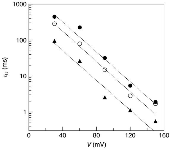
**Figure 7** Dependence of the characteristic unzipping timescale on the voltage measured using DVC, for 10 bp, 9 bp (10 bp with a mismatch), and 7 bp DNA hairpins (solid circles, empty circles, and triangles, respectively). As a first approximation, all molecules follow a monoexponential dependence on  $V$  with the same slope. (Reproduced with permission from Ref. 19).
