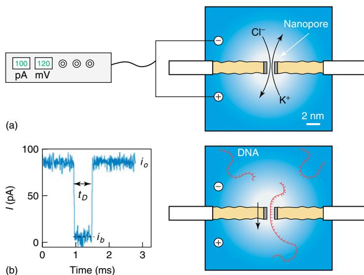
**Figure 1** The nanopore method: (a) The ion current flowing through a single-nanoscale pore is measured using a pico-ampere electrometer. (b) The insertion and threading of biopolymers cause abrupt blockades in the ion current, during the time in which the molecules remain in the pore. An electrical field applied across the membrane results in a strong force, driving the charged biopolymers from the negative to the positive chambers.
