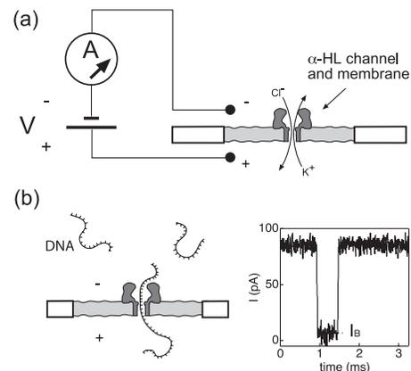
FIG. 1.  $I$ - $V$  measurements (a) for an “open” pore, and (b) when single-stranded DNA is electrophoretically threaded through the pore. DNA abruptly blocks the ion current from 80 pA to  $\sim 7$  pA ( $I_B$ ), as shown in the inset ( $C = 1$  M KCl,  $V = 120$  mV,  $T = 8^\circ\text{C}$ ).
