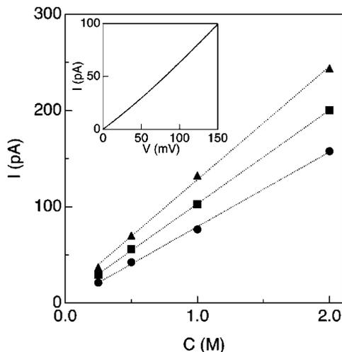
FIG. 2. Open pore current characteristics at  $T = 8^\circ\text{C}$ . The main figure displays the dependence of the current on the bulk KCl concentration measured at 120, 150, and 180 mV (circles, squares, and triangles, respectively). Lines are linear regression fits. The inset is the measured  $I$ - $V$  at 1 M KCl.
