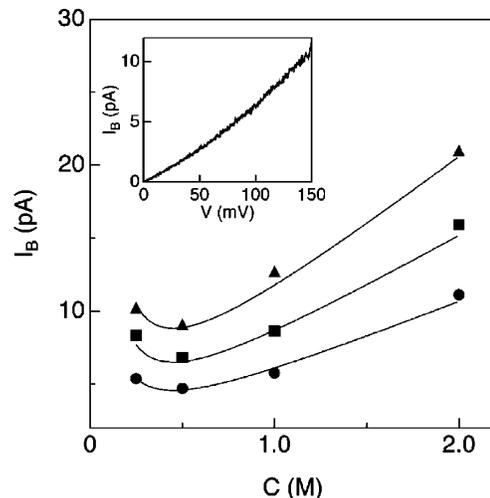
FIG. 3. Main figure: The dependence of the blocked ion current,  $I_B$ , on bulk ion concentration measured at 120, 150, and 180 mV (circles, squares, and triangles, respectively).  $I_B$  values were determined from the peak of the distributions of  $>1000$  DNA translocation events for each  $C$  and  $V$ . Solid lines are guides to eyes. The inset displays the measured  $I$ - $V$  curve for the blocked pore, performed using dynamic voltage control [5,14].
