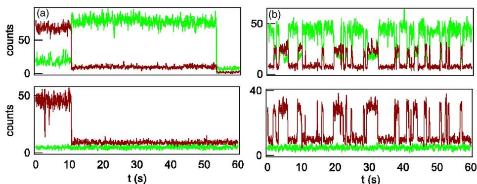
FIG. 3. Representative time traces of individual DNA molecules internally labeled with TMR and Cy5 fluorophores excited using alternating green and red lasers (0.5 and 0.13 kW/cm<sup>2</sup>, respectively). (a) TMR-6-Cy5 during green (top panel) and red excitations (bottom panel). (b) TMR-14-Cy5 during green (top panel) and red excitations (bottom panel). Note the perfect correlation between the acceptor emissions during green and red excitations.
