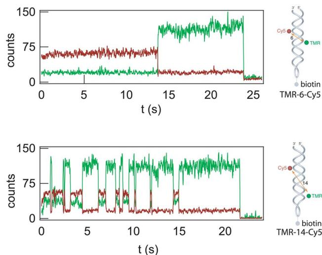
FIG. 1. Representative time traces of individual DNA molecules internally labeled with TMR and Cy5 fluorophores with an interdyne separation of six nucleotides (top panel) and 14 nucleotides (bottom panel). Schematics of the constructs are given to the right of the traces. The red lines correspond to counts (per 10 ms) from the acceptor channel and the green lines from the donor channel, excited by a 514 nm laser (0.5 kW/cm<sup>2</sup> at sample).
